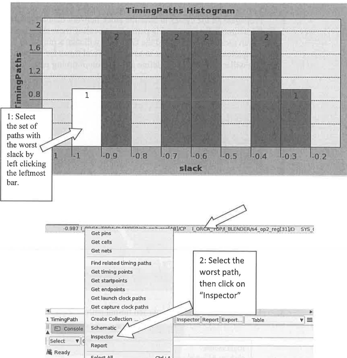
5. In the Path Inspector, examine clock reconvergent pessimism: In the data required and data arrival section, scroll down until you find CRP. Then, scroll across until you find the percent of delay for the CRP.
