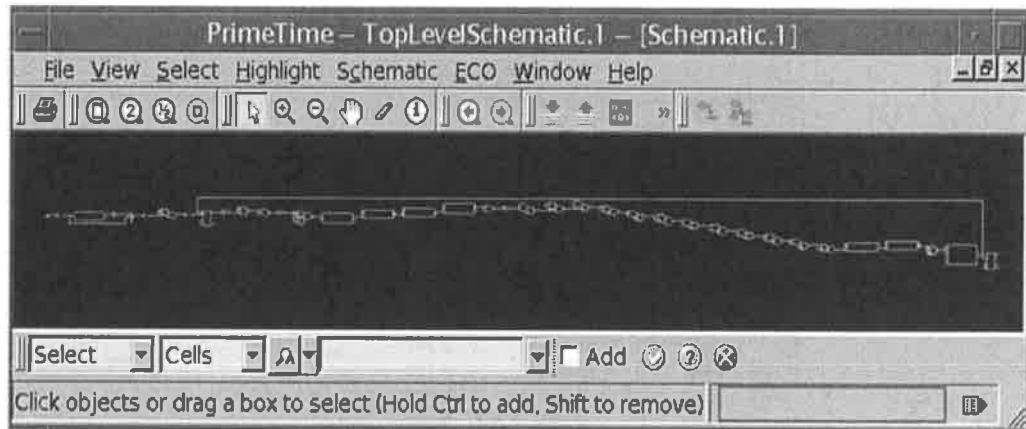
7. In the schematic window, find the CRP (clock reconvergent pessimism) point. This is the last pin before the launch and capture paths diverge.
