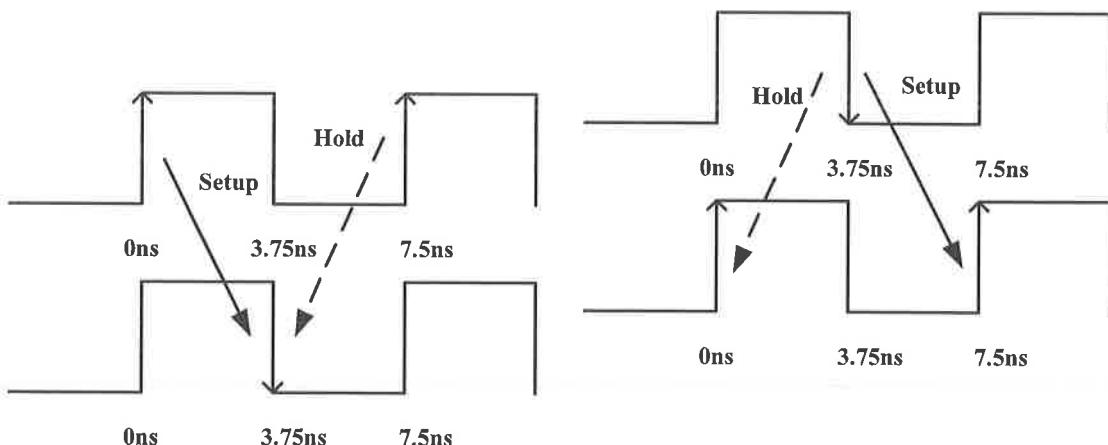
**Question 23.** For this same timing path, describe the specific clock edges that will be used in a timing report for hold timing checks.
